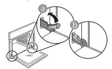
Apply gentle pressure to check that the catches are in the correct position.
