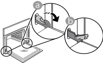
Simply remove the door by continuing to close it and at the same time lifting it until it comes out of its housing. Place the door on one side, supported on a soft surface.
