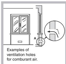
The air circulation system may take air directly from the outside by means of a pipe with an inner cross section of at least 100 cm<sup>2</sup>; the opening must not be vulnerable to any type of blockages.
