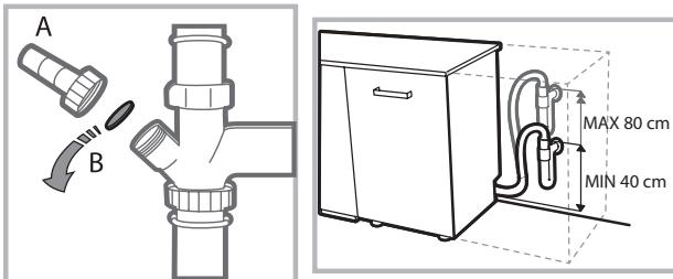
Before connecting the water outlet hose to the sink drain, remove the plastic plug (B).
