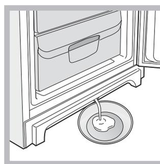
4. Certain appliances are fitted with the DRAIN SYSTEM to lead the water outside: let the water flow into a container (see diagram).
