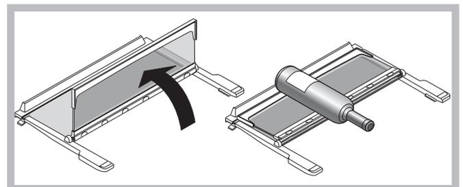
The central shelf of the fridge compartment folds on itself to create space for the bulky containers located on the shelf beneath it. For maximum flexibility in the use of internal space, the shelf can be positioned in place of other shelves according to the required need.
