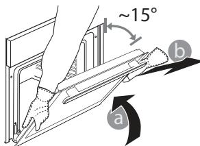
**Refit the door** by moving it towards the oven, aligning the hooks of the hinges with their seating and securing the upper part onto its seating.
