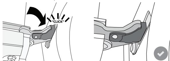
4. Try closing the door and check to make sure that it lines up with the control panel. If it does not, repeat the steps above: The door could become damaged if it does not work properly.
