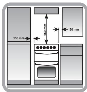
The height of the cooker can be adjusted by means of adjustable feet in the plinth (900mm - 915mm). Adjust the feet by tilting the cooker from the side. Then install the product into position. NOTE: This appliance must not be fitted on a platform.
