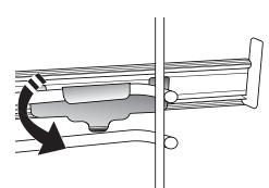
5. Repeat these steps on the other shelf guide on the same level. The sliding runners can be fitted on any level.
