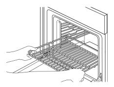
2. Other accessories, such as the drip tray and the baking tray, are inserted horizontally in the same way as the wire shelf.
