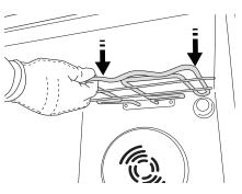
**4.** To reposition the heating element, lift it up, pulling it slightly towards you, be sure it comes to rest on the lateral supports.
