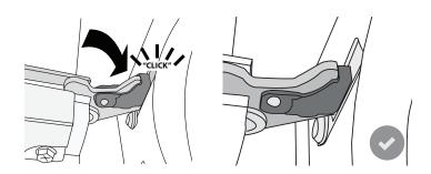
6. Try closing the door and check to make sure that it lines up with the control panel. If it does not, repeat the steps above: the door could become damaged if it does not work properly.
