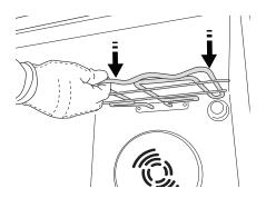
**4.** To reposition the heating element, lift it up, pulling it slightly towards you, be sure it comes to rest on the lateral supports.
