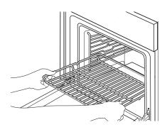
Other accessories, such as the drip tray and the baking tray, are inserted horizontally in the same way as the wire shelf.
