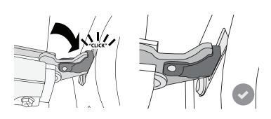
**6.** Try closing the door and check to make sure that it lines up with the control panel. If it does not, repeat the steps above: the door could become damaged if it does not work properly.
