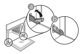
**5.** Apply gentle pressure to check that the catches are in the correct position.
