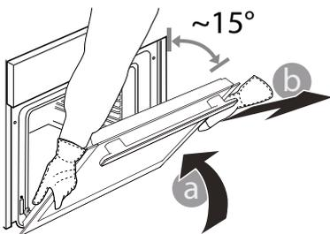
3. Refit the door by moving it towards the oven, aligning the hooks of the hinges with their seating and securing the upper part onto its seating.
