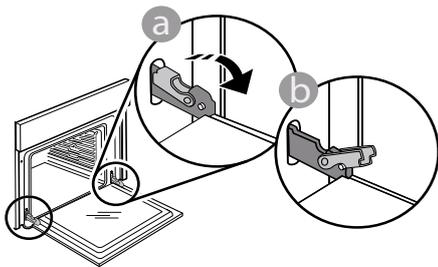
Simply remove the door by continuing to close it while pulling it upwards at the same time until it is released from its seating. Put the door to one side, resting it on a soft surface.
