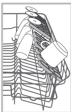
Wine glasses can be placed safely in the tip-up compartments by inserting the stem of each glass into the corresponding slots.
