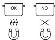
Only use pots and pans made from ferromagnetic material which are suitable for use with induction hobs. To determine whether a pot is suitable, check for the
