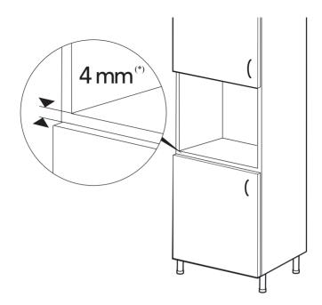
(\*) If the cabinet has a door at minimum distance of 4mm from the support surface, add the feet and relative 1mm washers, supplied in the packaging, on the bottom.
