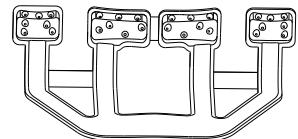
The lower rack has a Space Zone, a special pull-out support in the rear of the rack that can be used to support frying pans or baking pans in upright position, thus taking up less space.
