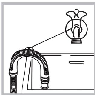
Alternatively, place the drain hose over the edge of a washbasin or bathtub, by fastening the guide
