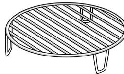
This allows you to place food closer to the grill, for perfectly browning your dish and for optimal hot air circulation. Place the wire shelf on the turntable, making sure that it does not come into contact with other surfaces.
