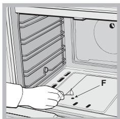
To light the oven burner, bring a flame or gas lighter close to opening F (see figure) and press the OVEN control knob while turning it in an anticlockwise direction until it reaches the MAX position.
