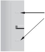
**In some models:** while loading the freezing compartment, do not load above the loading lines otherwise the door may not close correctly.
