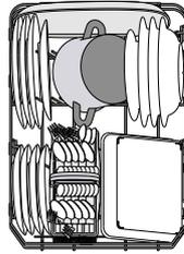
For pots, lids, plates, salad bowls, cutlery etc. Large plates and lids should ideally be placed at the sides to avoid interferences with the spray arm.
