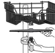
To remove the upper spray arm, turn the plastic locking ring in a clockwise direction.
