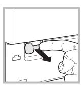
4. pull outwards using the tab as indicated in the figure, until the plastic tie-rod is freed from its stop position; pull downwards and open the door at the same time.
