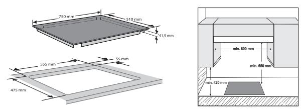
NOTE: if distance "A" between the kitchen cabinets is between 600 mm and 750 mm, height "B" must be at least 530 mm. If distance "A" between the kitchen cabinets is greater than the width of the hob, height "B" must be at least 400 mm. If a hood is installed above the hob, refer to the assembly instructions for the hood to see the necessary distance.
