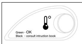
The temperature indicator is located on the bottom right hand side of the refrigerator wall. This indicator shows when the refrigerator compartment of your larger fridge is operating at the correct temperature.
