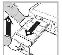
! Failure to empty the water container will cause the machine to stop heating and the load may still be wet at the end of the drying cycle. The 'Empty Water' light will tell you that the water container needs to be emptied
