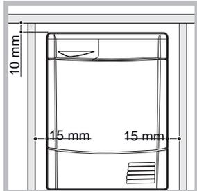
Install the dryer far from gas ranges, stoves, radiators or hobs as flames may damage it. If the dryer is installed below a worktop, ensure there are 10 mm between the upper panel of the dryer and any objects above it and 15 mm between the sides of the machine and the walls or
