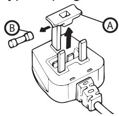
1. Remove the fuse cover (A) and fuse (B).
