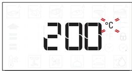
When the °C/°F icon flashes on the display, turn the knob to change the value, then press to confirm and continue to alter the settings that follow (if possible).
