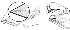
**4.** Refit the upper edge: a click will indicate correct positioning. Make sure the seal is secure before refitting the door.
