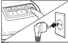
Before removing the pitcher from the base, always press POWER ((1)) to stop the flashing lights and unplug the power cord.
