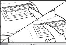
Press POWER ((1)). The Power indicator light will flash when ready. Then press desired speed button for continuous operation at that speed. The white indicator light by the selected speed will stay lit. You may change settings without stopping by pressing a new speed button.
