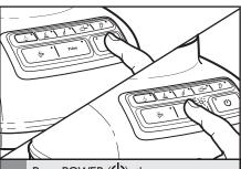
Press POWER ((1)), then press PULSE (\*Pulse\*). The indicator lights above the Pulse button and all four speeds will blink to indicate that all four speeds are in the PULSE (\*Pulse\*) mode.
