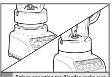
Before operating the Blender, make sure the pitcher is properly positioned on the base.
