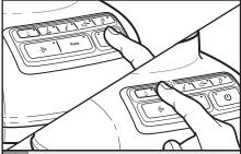
Press and hold a speed button for the desired length of time. Both the speed button and PULSE mode indicators will stay lit when pulsing. Blending will stop when Pulse button is released and the Pulse indicator will resume blinking. To pulse again at another speed, just press and hold the desired speed button.
