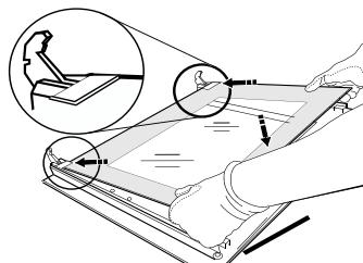
**4.** Refit the upper edge: a click will indicate correct positioning. Make sure the seal is secure before refitting the door
