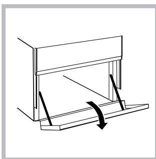
There is a compartment underneath the oven that may be used to store oven accessories or deep dishes. To open the door pull it downwards (see figure).
