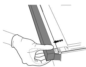
**2.** Lift and firmly hold the inner glass with both hands, remove it and place it on a soft surface before cleaning it.
