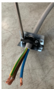
Fix power cord to the plastic holder.
