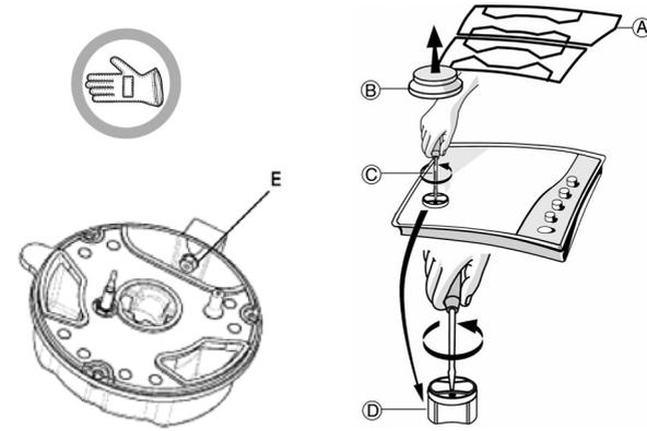
Before installing the hob, remember to affix the gas calibration plate supplied with the injectors in such a way that it covers the existing information relating to gas calibration.
