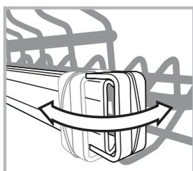
Release the two locks (right and left) and pull out the rack. When the upper rack is fitted, the locks must be always closed.
