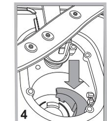
After cleaning the filters, re-place the filter assembly and fix it in position correctly; this is essential for maintaining the efficient operation of the dishwasher.
