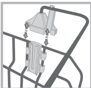
Before loading the tray, make sure the supports are properly coupled to the upper rack (see Figure).
