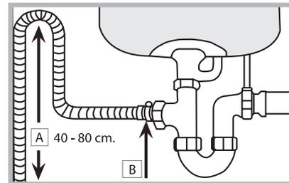
Before connecting the water outlet hose to the sink drain, remove the plastic plug (B).
