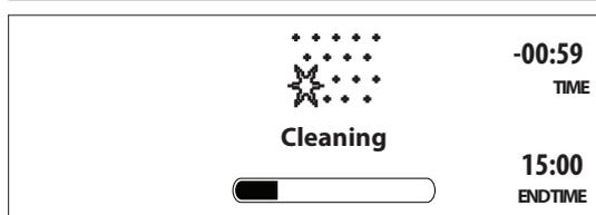
A message will start flashing on the display once the cycle has finished. The residual temperature will be indicated on the display and the door will remain locked until the temperature inside the oven has returned to a safe level. The display will then show the current time.
