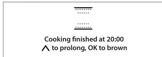
If required, press **OK select** to activate a five-minute browning cycle. It is also possible to extend the cooking time while maintaining the active function by pressing **▲**.
