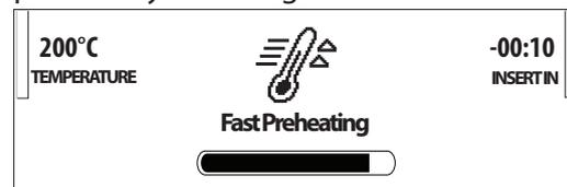
Once preheating has finished, an audible signal will sound to indicate that the oven has reached the set temperature. At this point, place the food in the oven and begin cooking by pressing **▷**: the oven will automatically select the Conventional function. If you wish to set a different cooking function, press **MENU** and select the desired function.
