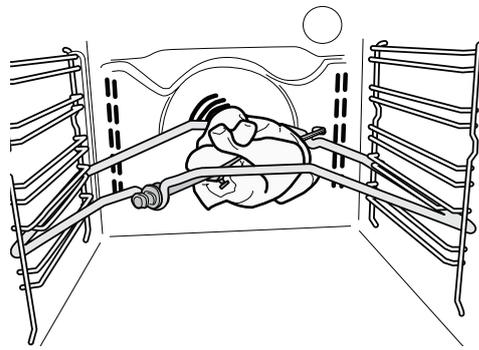
To use the turnspit, select the "Turbo grill" function. To collect the cooking juices, position the drip tray below the meat and add 500 ml of water.
