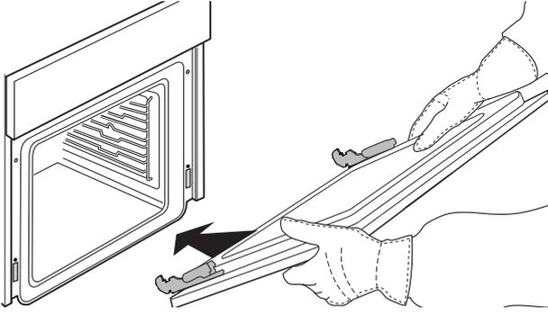
5. Apply gentle pressure to check that the catches are in the correct position.
