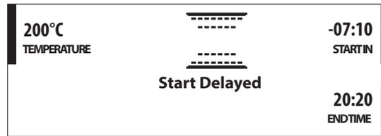
To activate the function immediately, cancelling the programmed delay time, press **▷**.
