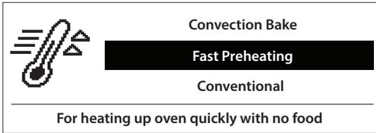
Press **▲** or **▼** to navigate through the list given. Press **OK select** to confirm and go to the Settings menu: The display will show the basic settings for the function.
