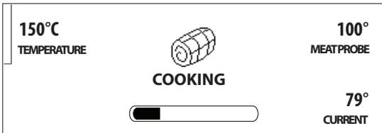
An audible signal will sound and the display will indicate when the food probe has reached the required temperature. Once cooking is complete, the result can be perfected by extending the cooking time. Press **▲** or **▼** to set the length of time: the oven will use the Conventional function automatically.
