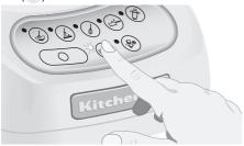
4. Select a speed button. Press and hold for the desired length of time. Both the speed button and PULSE (Pulse) mode indicators will stay lit when pulsing at the selected speed. When button is released, the blending will stop, but the Blender will remain in PULSE (Pulse) mode and the PULSE (Pulse) mode indicator will return to blinking. To pulse again or at another speed, simply press and hold the button of the desired speed.
