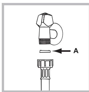
1. Insert seal A into the end of the inlet hose and screw the latter onto a cold water tap with a 3/4 gas threaded mouth (see figure). Before making the connection, allow the water to run freely until it is perfectly clear.
