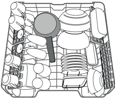
The upper rack has tip-up supports which can be used in a vertical position when arranging tea/ dessert saucers or in a lower position to load bowls and food containers.
