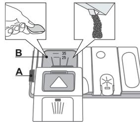
**To open the detergent dispenser use the opening device A. Introduce the detergent into the dry dispenser B only. Place the amount of detergent for pre-washing directly inside the tub.**
