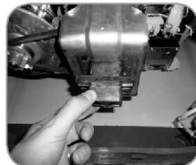
The opening on the base must not be obstructed by a carpet.
