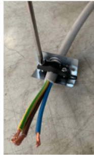
Fix power cord to the plastic holder.
