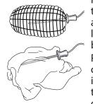
Insert the food probe deep into the meat, avoiding bones or fatty areas. For poultry, insert the probe lengthways into the centre of the breast, avoiding hollow areas. Place the food in the oven and connect the plug by inserting it into the connection provided on the righthand side of the oven's cooking compartment.
