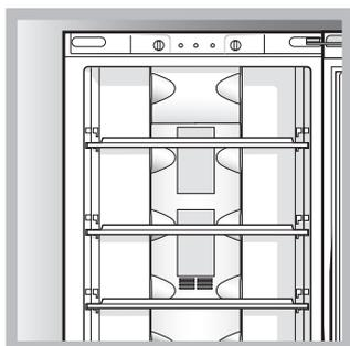
It is recognisable by aeration cells located on the back walls of the compartments. The No Frost system circulates cold air continuously to collect humidity and prevent ice and frost formation. The system maintains an optimal humidity level in the compartment, preserving
