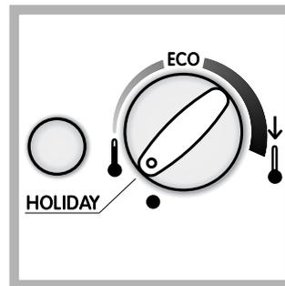
To enable the function: set the REFRIGERATOR OPERATION knob on **HOLIDAY** (see diagram). A double acoustic signal informs you when it has been enabled. A single acoustic signal informs you when it has been disabled.
