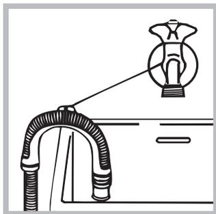
Alternatively, place the drain hose over the edge of a washbasin or bathtub, by fastening the guide (which can be purchased at the technical assistance centre) to the tap (see figure). The free end of the hose should not be
