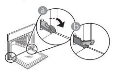
Simply remove the door by continuing to close it while pulling it upwards at the same time until it is released from its seating. Put the door to one side, resting it on a soft surface.
