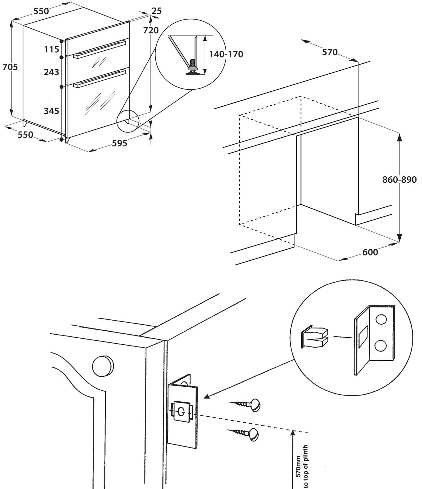
A minimum distance of 25mm should be maintained between the front face of the cabinet side and the front face of the plinth.
