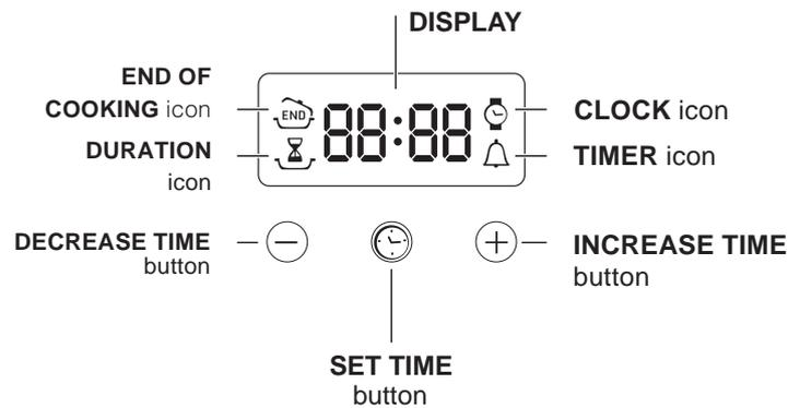
The Top Oven and Bottom Oven can be controlled by the automatic timer. When the timer control has been set for one oven, it is possible to use the other oven only during the same automatic cooking programme.
