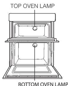
Disconnect the oven from the power supply. Unscrew the cover from the light, replace the bulb (25W - 230V - T 300 °C - E14) and screw the cover back on the light. Reconnect the oven to the power supply.
