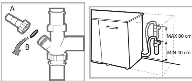
Before connecting the water outlet hose to the sink drain, remove the plastic plug (B).
