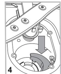
After cleaning the filters, re-place the filter assembly and fix it in position correctly; this is essential for maintaining the efficient operation of the dishwasher.
