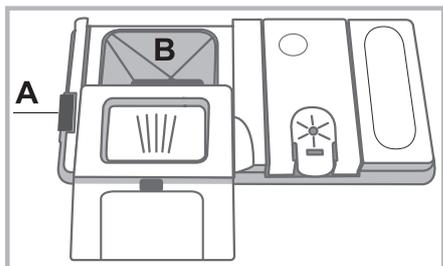
Introduce the detergent into the dry dispenser "B" only. Place the amount of detergent for pre-washing directly inside the tub.
