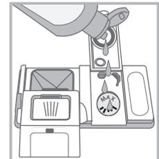
1. Open the dispenser "D" by pressing and pulling up the tab on the lid;
