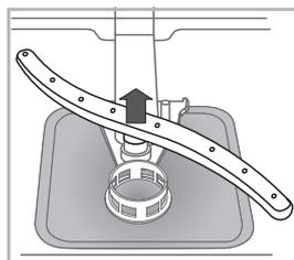
The lower spray arm can be removed by pressing on the side tabs and pulling it upwards.
