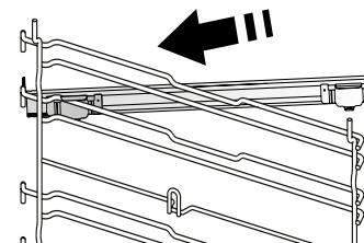
Fasten the upper clip of the runner to the shelf guide and slide it along as far as it will go. Lower the other clip into position.
