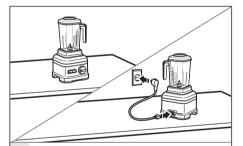
Before using the Blender, be sure the countertop beneath the Blender and surrounding areas are dry and clean. Then, plug the Blender into an earthed outlet.
