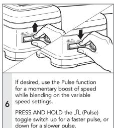
**NOTE:** The Pulse function  $\Lambda$  may also be used on its own as a separate blending function while the Blender is in Standby mode.
