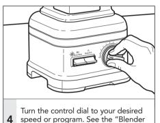
NOTE: If you select a preprogrammed cycle, you will need to flip the ▷II (Start/Stop) toggle to begin operation. The Blender will automatically stop running once the cycle is complete.
