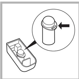
When pouring in the bleach, be careful not to exceed the "max" level marked on the central pivot (see figure).
