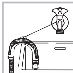
Alternatively, place the drain hose over the edge of a washbasin or bathtub, by fastening the guide hook (which can be purchased at the technical assistance centre) to the tap (see figure). The free end of the hose should not
