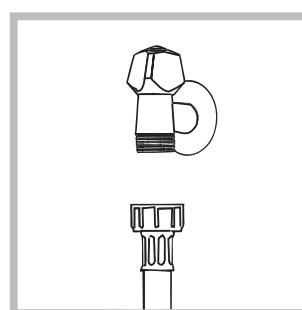
1. Connect the supply pipe by screwing it to a cold water tab using a  $\frac{3}{4}$  gas threaded connection (see figure). Before performing the connection, allow the water to run freely until it is perfectly clear.
