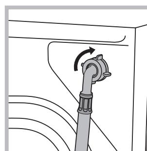
2. Connect the inlet hose to the washing machine by screwing it onto the corresponding water inlet of the appliance, which is situated on the top right-hand side of the rear part of the appliance (see figure).
