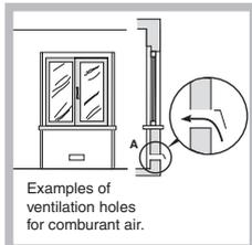
Examples of ventilation holes for comburant air.
