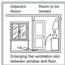
Enlarging the ventilation slot between window and floor.
