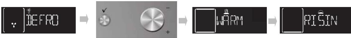
1. Turn the "Functions" knob to symbol : the display shows "DEFROST" along with this function's corresponding symbol.
