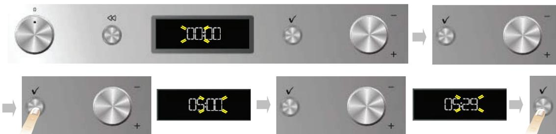
After connecting the oven to the mains power, the time must be set on the clock. The two hour digits flash on the display.
