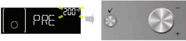
1. Turn the "Functions" knob to the symbol
