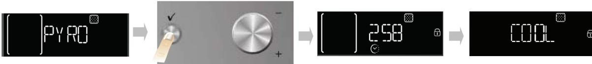
To activate the oven's automatic cleaning cycle (pyro-cleaning), proceed as follows:
